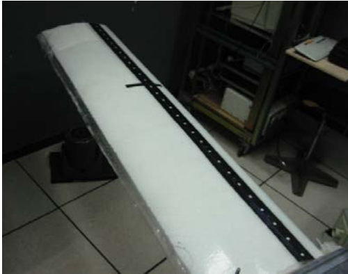
Figure 12a: Photograph of the wing. In white is the body of the wing, in black is the spar.
