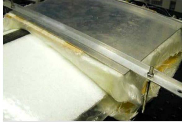
Figure 12b: Photograph of a detail of the clamped end of the wing.
