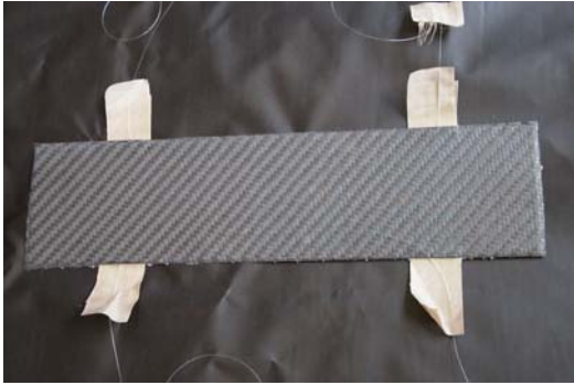
Figure 6: Teflon ribbon protecting the egress of optical fibres from a CFRP laminate.
